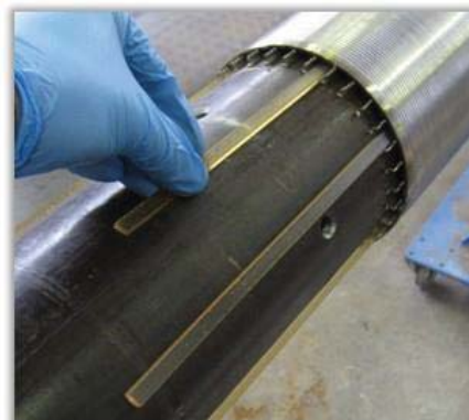
Fig. 2 RESMAN can be easily integrated into the completion components, eliminating design complexity and operational risk
